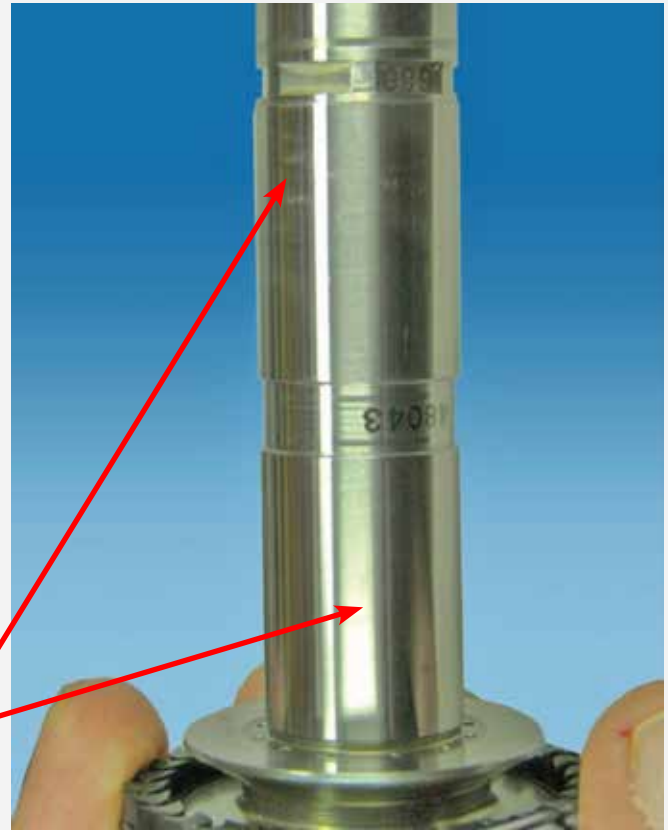
Figure 1-3: New Shaft Appearance
