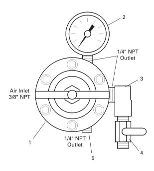
PARTS LIST - Model HAR-600 Regulator and Gauge Assembly
