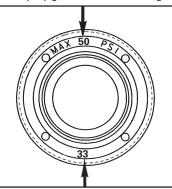
Air cap number located on face of capcap number must correspond with baffle number to assure 10 PSI cap pressure.
