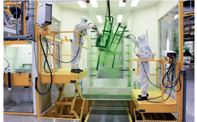
Flexible powder coating of flat and / or large work- pieces.
