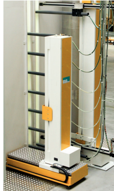
Automated coating with combination X-Y-Z axis controls.
