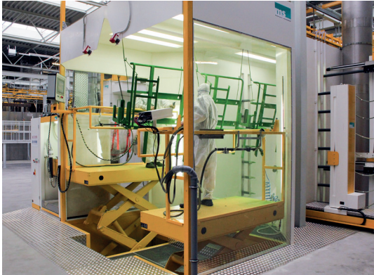
Manual coating area with integrated scissor lift tables.
