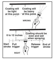
For best results, use 3 to 6 psi fluid pressure. Higher than 6 psi fluid pressure may be required for heavy-bodied materials. Low fluid pressures will produce a narrower than normal spray pattern. Generally use 30-35 psi air at gun inlet (see page 7). Unusually heavy, difficult to atomize fluids may require up to 50 psi air at gun inlet.
