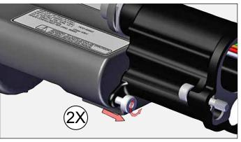
12. Remove internal housing screws.
