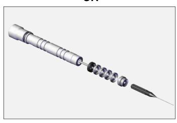
7. Insert packing tube onto shaft. Wipe excess grease over front parts and outside of packing tube.
