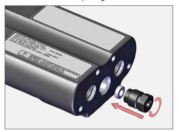
5. Install fluid inlet fitting.
