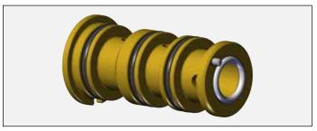
11. Install bushing into piston housing.
