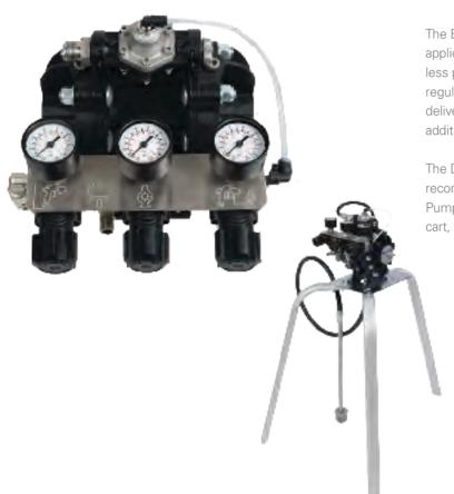
The Binks DX70 is the perfect solution for one gun spray applications with faster color changes and quick refills for less production downtime. The DX70 includes a built in fluid regulator which ensures a constant and virtually pulse free fluid delivery. The DX70 design reduces the cost and complexity of additional fluid regulators or surge chambers.
