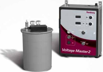
VoltageMaster2 is Ransburg's compact high voltage power supply, features full PLC remote control capability and is completely backwards compatible with a universal range of applicators and other systems. With its ability to produce up to 100kV DC continuous operating voltage while delivering up to 1,500 microamps load current, this is the workhorse power system for your finishing operation.
