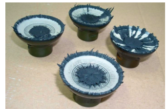
ICE-Bell 2's low operating temperature avoids contaminated bell cups like these.
