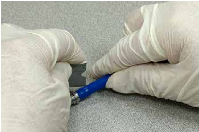
Cut tube from barb and remove tubing.
