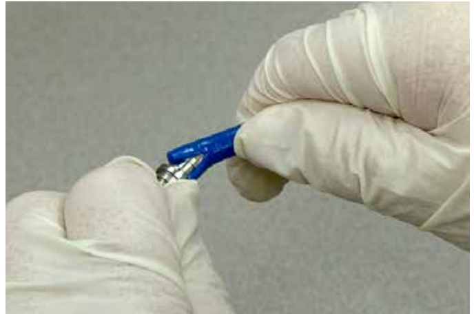
Cut off damaged tubing and follow installation instructions.
