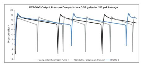
The 'longer—slower' cycle rate of the DX200-3 moves the same volume of fluid but at a slower cycle rate than its competitors. This means less stress and wear on components, resulting in longer intervals between maintenance inspections.
